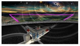
Einstein Telescope will achieve a greatly improved sensitivity by increasing the size of the interferometer from the 3km arm length of the Virgo detector to 10km, and by implementing a series of new technologies. These include a cryogenic system to cool some of the main optics to 10 - 20K, new quantum technologies to reduce the fluctuations of the light, and a set of infrastructural and active noise-mitigation measures to reduce environmental perturbations.
