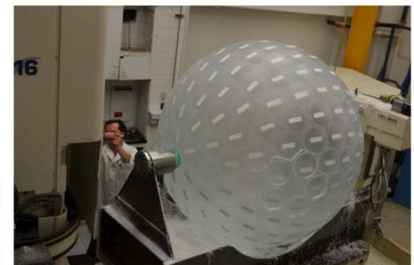
DEAP Acrylic Vessel with Light Guide "Stubs" July 2012
