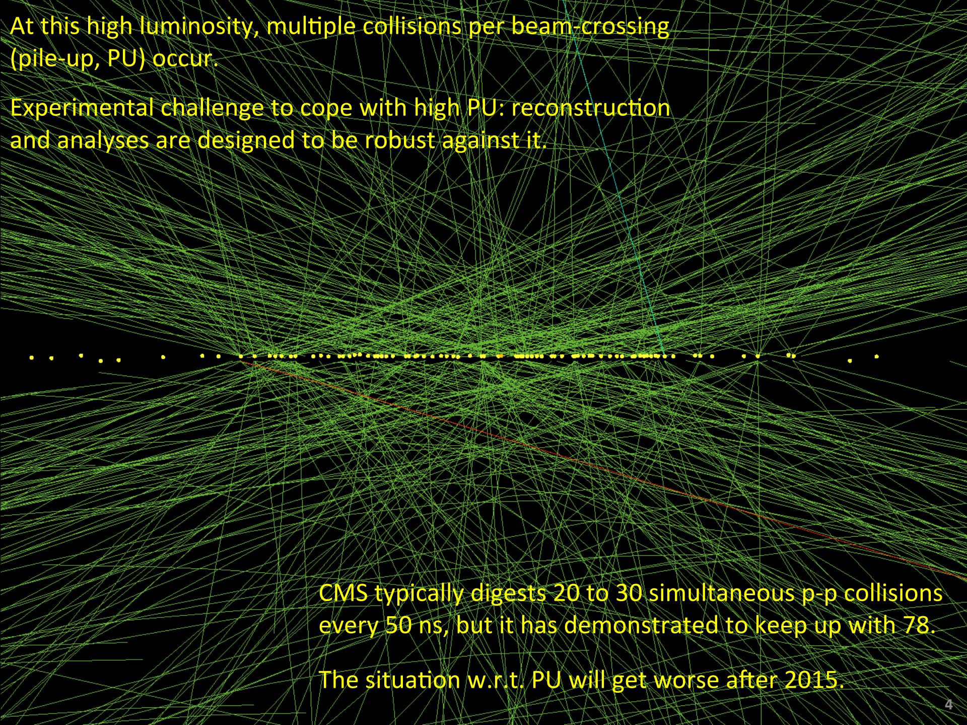
CMS typically digests 20 to 30 simultaneous p-p collisions every 50 ns, but it has demonstrated to keep up with 78.
