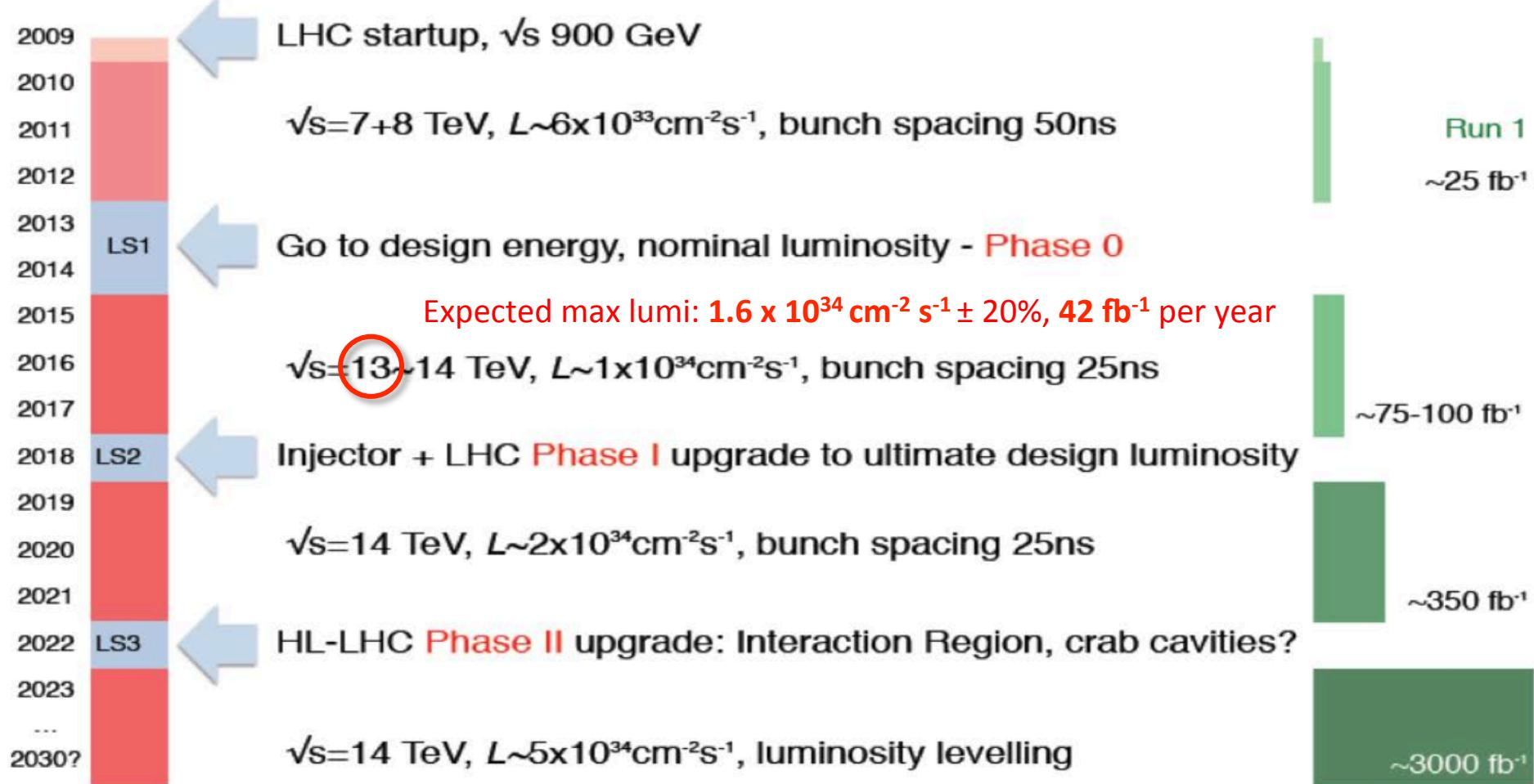
LS1: complete muon coverage (ME4), improve muon trigger, DT electronics, replace HCAL photo-detectors in Forward (new PMTs) and Outer (HPD $\rightarrow$ SiPM)
